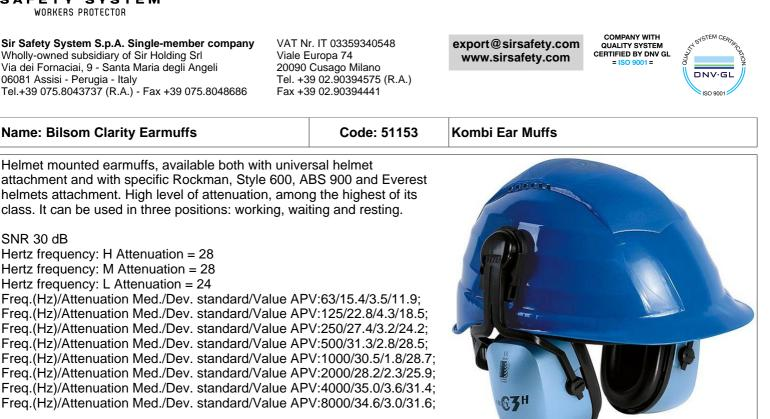
The product is designed and manufactured to comply with the essential health and safety requirements of Directive 89/686/EEC, and to conform to the requirements of EN 352. It is classified as PPE Cat. II.
